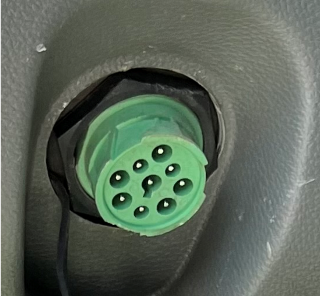
Figure 2. 9-pin OBD connector used for J1939
